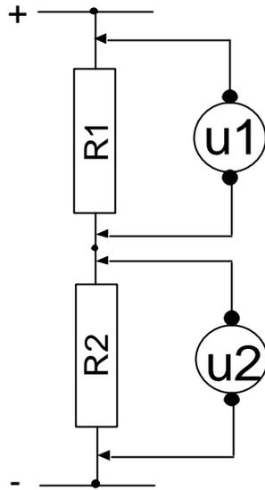
$$U_1 = U_{\text{tot}} \times \frac{R_1}{R_1 + R_2}$$
